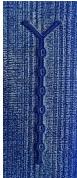
Figure 6: Fabricated microchannel or mold with Elliptical Obstacles
